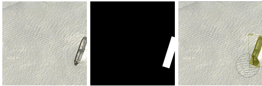
Figure 9. Airbus Ship Detection dataset ground truth annotation example. Left: original image; Middle: ground truth annotation mask. Right: magnified detail showing the discrepancy between the mask and the true ship segmentation.
