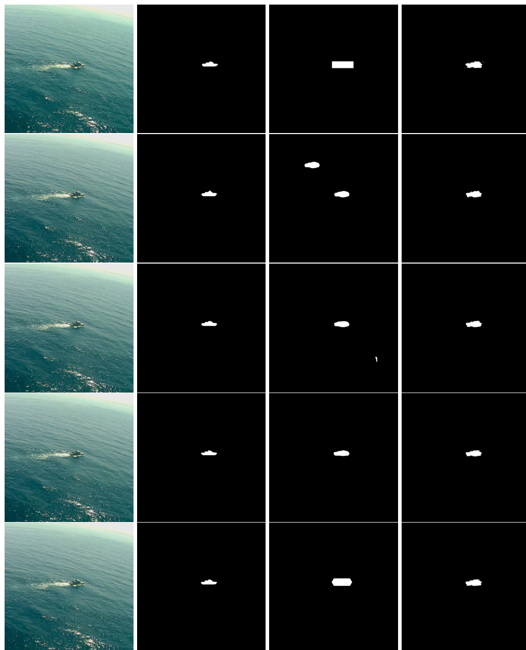
Figure 13. Simulating incorrect Yolact++ segmentations on the Seagull dataset. First rows correspond to older images, while the bottom row corresponds to the most recent image frame. First column: original images; second column: ground-truth annotations; third column: Yolact++ manually disturbed segmented images; fourth column: final segmentation result after post-processing with the 3D CRF.
