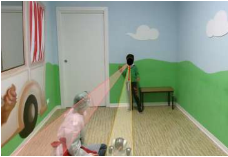
Fig. 1. Representation of the attention classification system, where the Therapist (pink cone) and NAO (yellow cone) areas of interest are compared with the subject gaze direction estimation (red arrow). In this case the system would classify as 'looking at the robot'.
