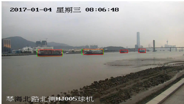
Fig. 6. Example of detections in the Seaships dataset [25]. In green, annotations, in red, detections.
