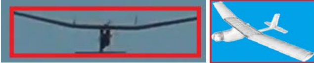
Figure 3. Example of object inner (object) and outer (between the object and the bounding box) regions where color histograms are computed for the particle likelihood metric.
