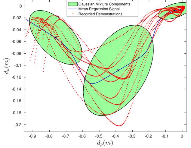
Fig. 4: Learned CDS between “giver” and “receiver”.  $d_p$  is the distance between wrists, parallel to the floor, and  $d_h$  is the difference of height, perpendicular to the floor, between wrists. The origin is when the wrists are at the nearest distance from the two which it is considered as the handover location.
