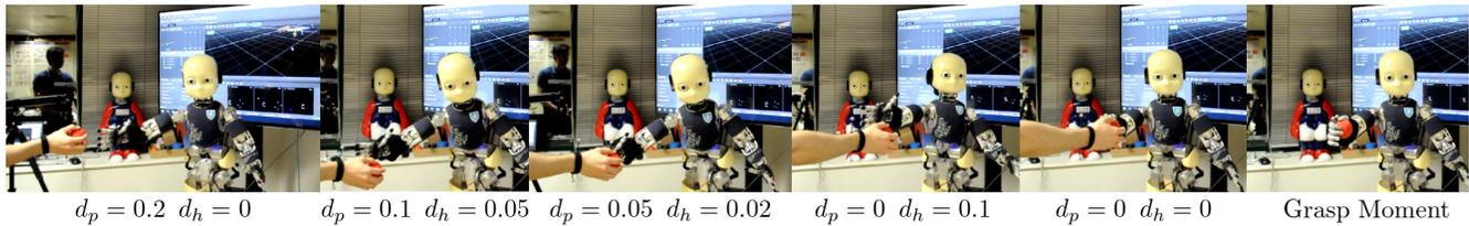
Fig. 7: HRI scenario of a handover action using the controller for coupling of arm movements. Below each specific moment it is represented the values for  $d_p$  and  $d_h$  which depending on the learned CDS it invokes a particular relation between the “giver” and “receiver”.
