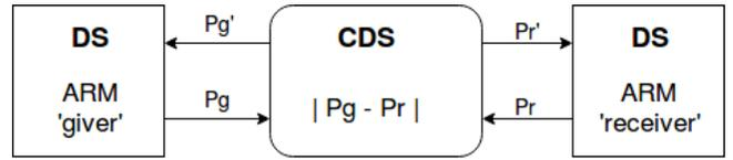
Fig. 3: Schematics of the Coupling of Arm Movements.  $P_g$  and  $P_r$  are the wrist position of the “giver” and “receiver”, respectively.  $P_g'$  and  $P_r'$  are the computed estimated wrist position of “giver” and “receiver”, respectively, from the coupling function in the next iteration.
