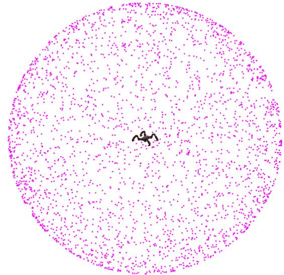
**Figure 4.** Robot and coverage sphere. In our sensor placement algorithm we optimize the number of viewing directions covered by the sensors, represented by the fraction of points visible on the surface of a large sphere.
