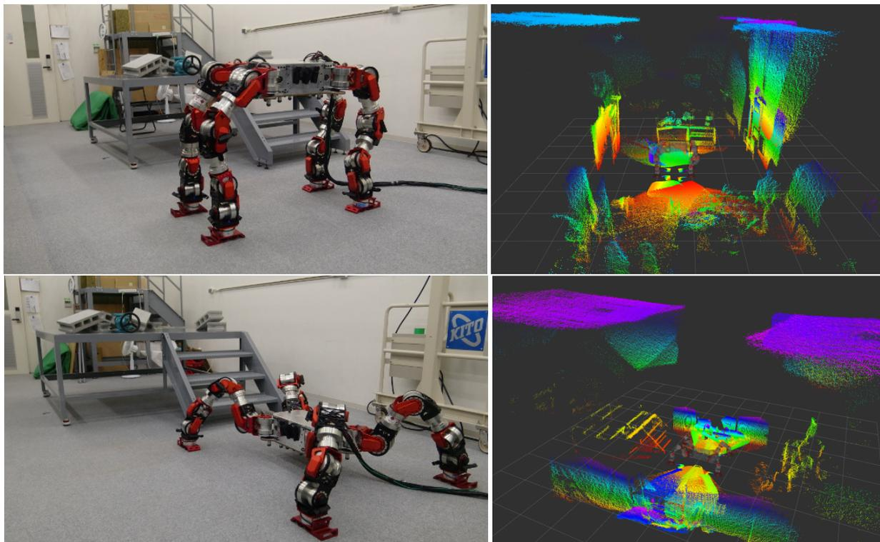
**Figure 10.** Point clouds of the full sensor system, when all sensors are acquired simultaneously (no scheduling). Top: quadruped, bottom: crawling locomotion.
