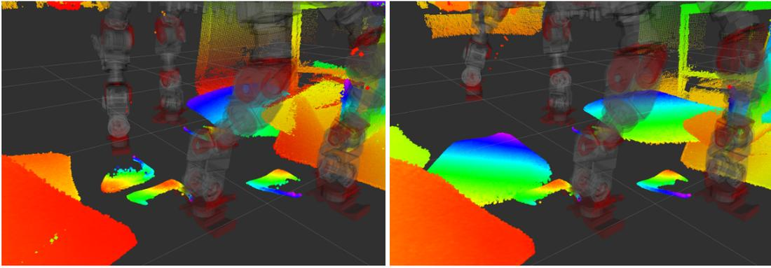
**Figure 11.** Simultaneously acquired point clouds, during quadruped locomotion. Left: all feet are in contact. Right: the robot lifts the forward-left foot before contacting the floor again. Coverage of the contact area increases while the leg is lifted.
