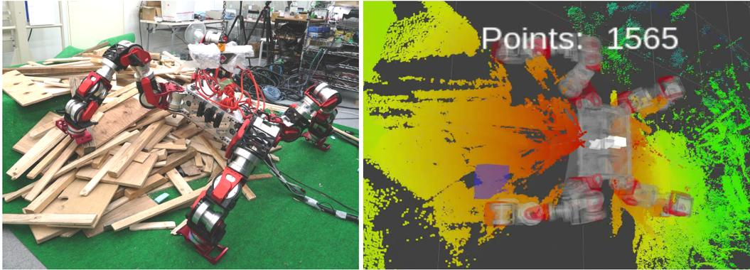
**Figure 12.** Point cloud density at the next contact point (task-specific coverage).
