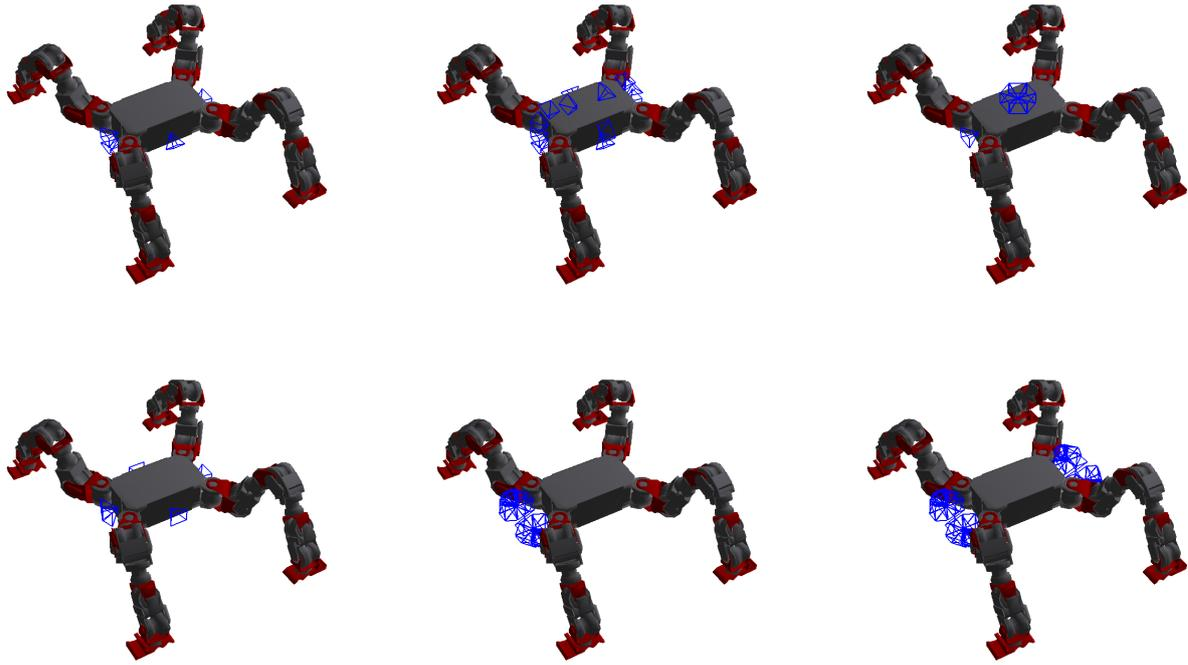
**Figure 5.** Design approaches used for comparison. From left to right, top to bottom: robosimian, robosimian-dbl, spotmini, spotmini-new, e2dr, e2dr-dbl.
