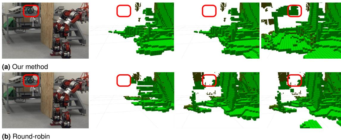
**Figure 22.** Evolution of the occupancy grid over time ( $t=3,7,11$ s) on the surprise-valve scenario. The red rectangle marks the object of interest, which is hidden behind a wooden wall at  $t=0$ . When walking past the wooden wall, our method quickly picks the previously-occluded viewing direction which reveals a valve (at  $t=11$ s) before the round-robin method does (at  $t=15$ s).
