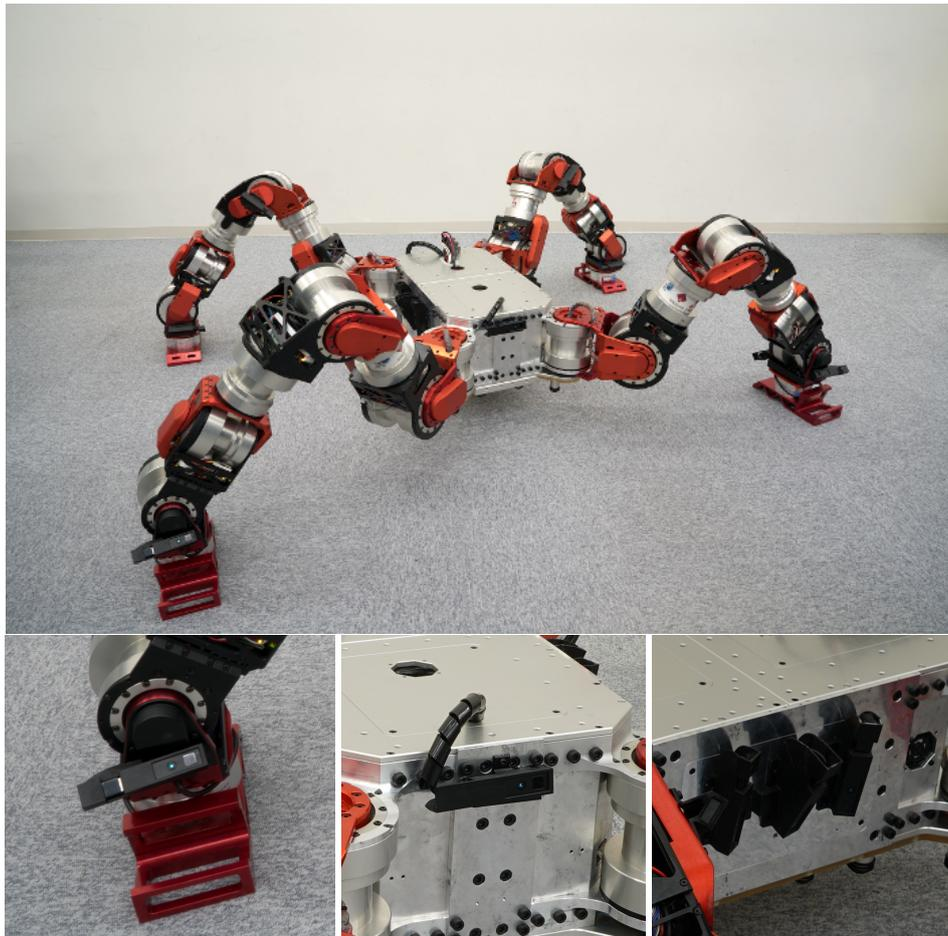
**Figure 9.** Final robot and a close-up of the camera holders.
