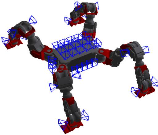
**Figure 3.** The set of 47 sensors used for optimization. Both sensor orientation and usage are optimized (i.e. roll-pitch-yaw angles and binary variables indicating whether each sensor is used in the final design or not).
