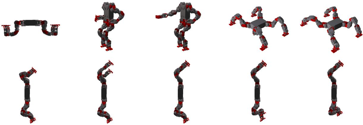
**Figure 2.** Robot configurations used for design optimization of the sensor system. From left to right, top to bottom: wheeled task (1 configuration), manipulation task (2), crawling task (2) and ladder-climbing task (5). In our experiments, each task as equal probability.
