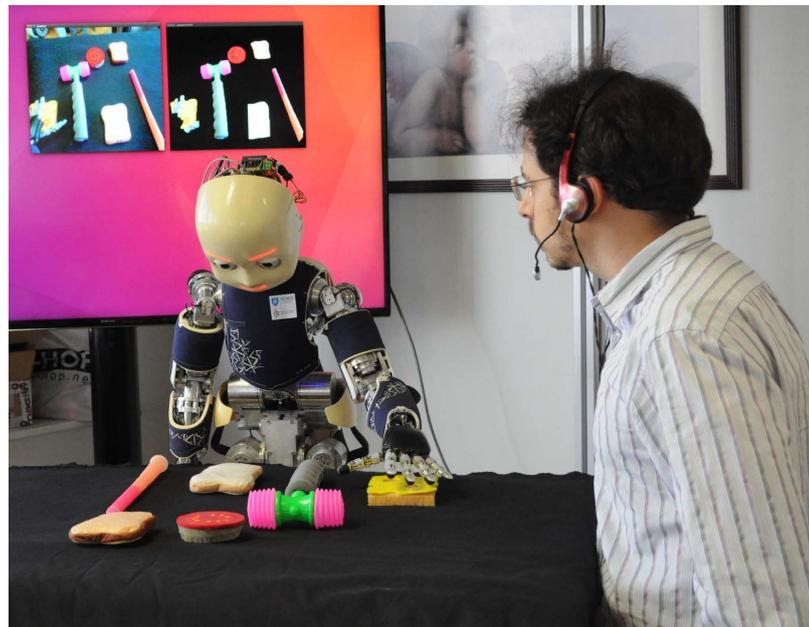
Figure 50: A robot performing a complex manipulation task after receiving a verbal instruction from a human. In the back screen, images from the robot cameras showing visual perception routines.
