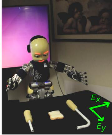
Figure 37: The iCub robot in a tool use scenario, with green overlay arrows showing the effects (i.e., displacements of objects).
