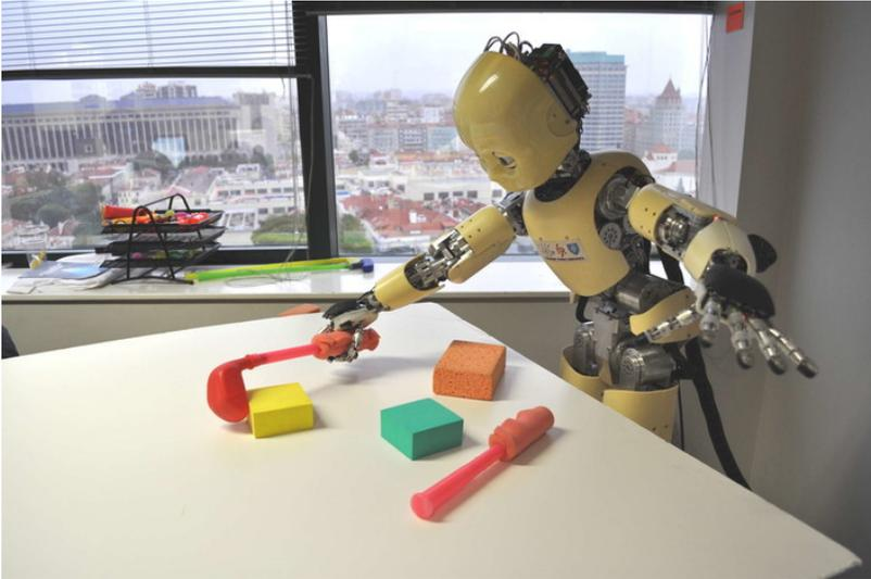
Figure 18: The iCub robot in a playground table scenario. Objects and tools are present in the scenario, so that the robot can interact with them, it can acquire a model of the environment derived from sensorimotor data, and it can use such a model for reasoning about the environment.
