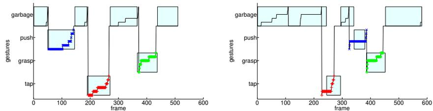
Figure 73: Gesture recognition VITERBI results on the early intention recognition scenario of Fig. 72 without noise. Red plus signs: tap states, green stars: grasp states, blue crosses: push states, rectangles: human-labeled ground truth segmentation.
