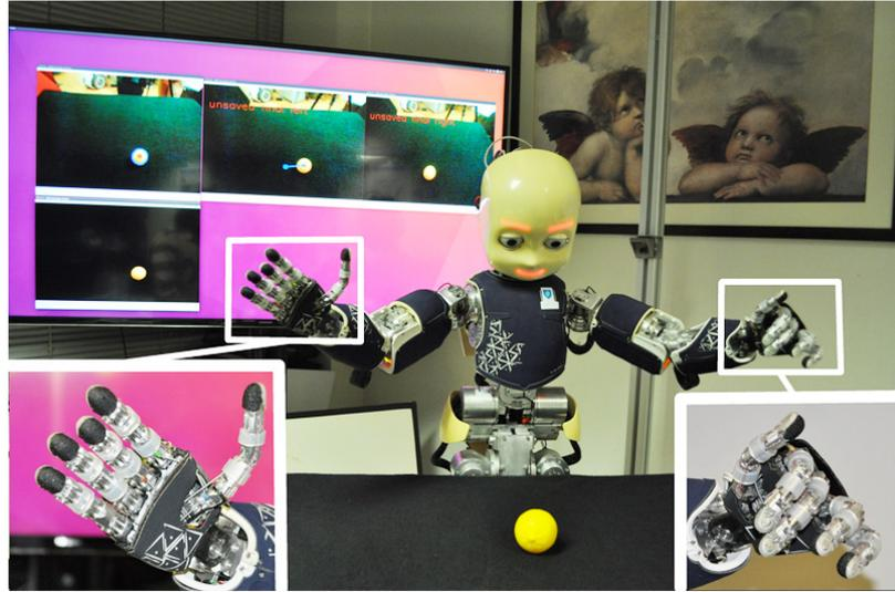
Figure 41: The iCub humanoid robot performing motor actions with different hand postures onto a physical object. In the background screen, we show the visual routines that monitor the evolution of the environment.
