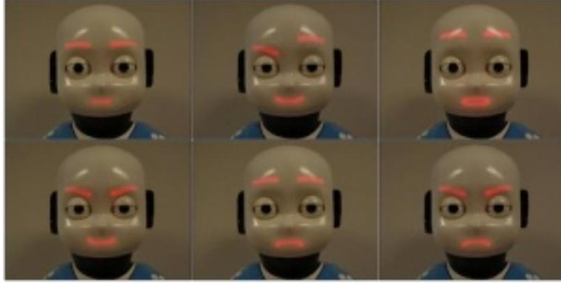
Figure 75: A set of iCub facial expressions using eye LEDs, mouth LEDs and eyelid motors.
