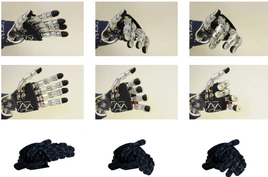
Figure 42: The three robot hand postures adopted to study the hand to tool transition. Left column: straight hand; center column: bent hand; right column: arched hand. The first two rows are real robot postures seen from different viewpoints; the last row shows the simulated body schema CAD model of the top viewpoint. From the latter simulated view, we obtain the segmented silhouette contour of the hand and its shape features.
