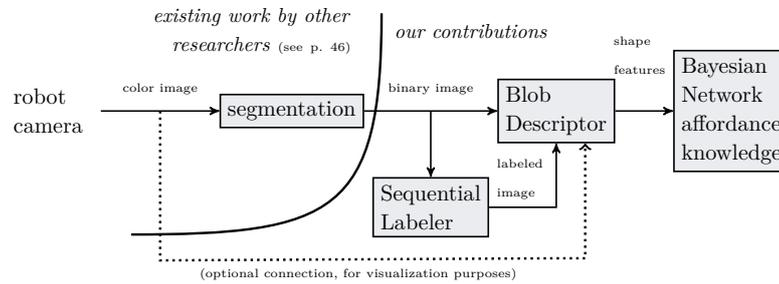
Figure 20: Our pipeline for computing visual affordance features. Boxes indicate software modules, arrows indicate data flow connections, dotted arrows indicate optional data flow connections. See text for details, and Fig. 21 for an example computation.
