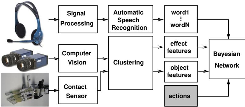
Figure 12: Experimental setup of [Sal+12]. In this work, which extends [Mon+08], a robot learns associations between *spoken words* and object affordances (where affordances are modeled as the relationships between actions, object features, effect features).
