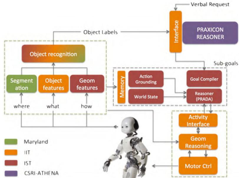
Figure 62: POETICON++ project software architecture. The contributions by IST are marked in red.
