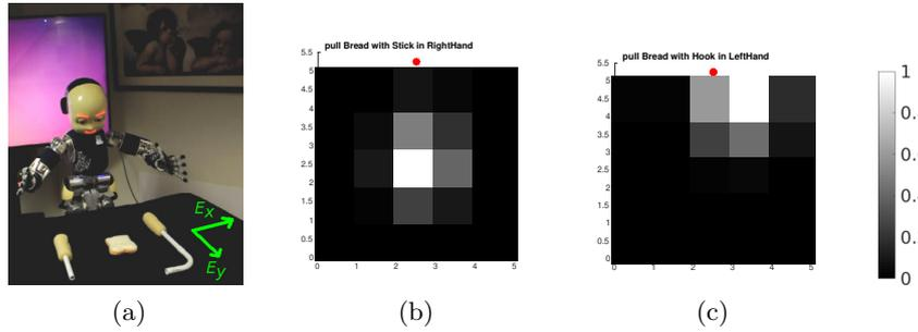
Figure 46: (a): the iCub robot using affordance reasoning to select the most appropriate tool for achieving a given action, i.e., pulling the bread closer to the agent. (b–c): effect prediction probabilities of the bread motion using the tools, where the robot location is marked with a red dot, and the table area is divided into a grid of squares.
