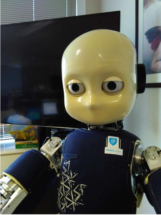
Figure 76: The iCub face in a neutral position, without facial expressions, as it was used during the human study of Sec. B.2.
