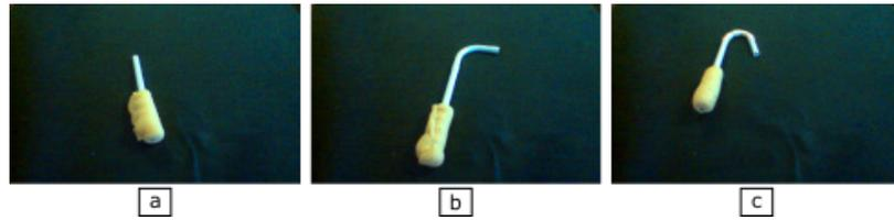
Figure 48: Hand to tool transition: the three baseline tools used in [Deh+16a], (a) stick, (b) rake and (c) hook. They provide different affordances when grasped by the hand of the robot and employed for performing motor actions onto objects. In this chapter, we consider these tool affordances as a comparison term to assess our novel hand affordances.
