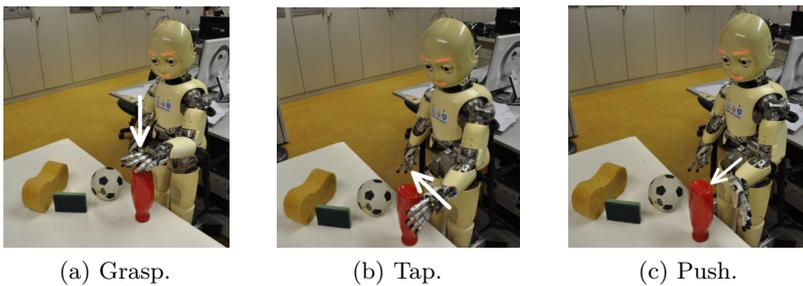
Figure 19: Examples of manipulative motor actions performed by the iCub robot onto environment objects.
