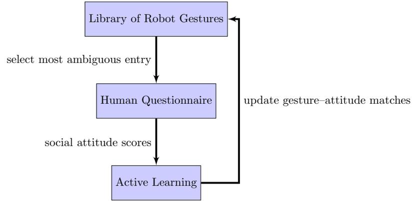
Figure 77: Block diagram of the proposed approach to study the matches between robot gestures and perceived social attitude in humans. The library of gestures is pre-programmed (see Table 18); the questionnaire is a multiple-scale Likert one; the scores are numbers corresponding to the Likert answers, and they are used by the Active Learning block to update an internal matrix of matches and select which robot gestures should be shown next.
