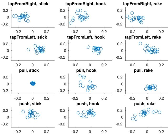
(b) Motion caused with *tools* when using different actions and tool types, taken from [Deh+16a]. Here we show only the interactions with 2 objects, to be consistent with Fig. 47a.
