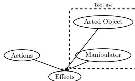
Figure 32: Computational model of affordances for dealing with multiple objects and tool use. In this chapter, the manipulator corresponds to the held object (i.e., tool) or to the robot hand.
