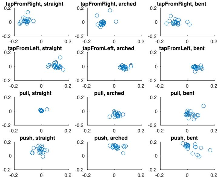
(a) Motion caused with the robot *hands* when using different actions and hand postures, as observed when interacting with 2 objects multiple times in our experiments.
