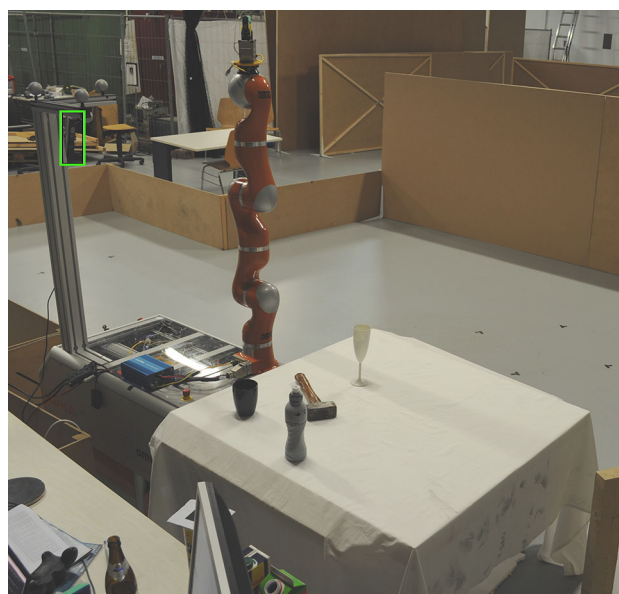
Fig. 11 The table is in front of the mobile platform. The range sensor is marked by the green rectangle
