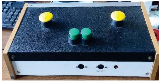
Figure 5.3: Board for tapping test
