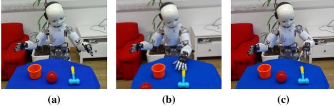
**Figure 5:** Snapshots of the iCub performing different exploration actions: a) looking at the hammer; b) pointing at the hammer and asking the label; and c) displacing the hammer on the table.
