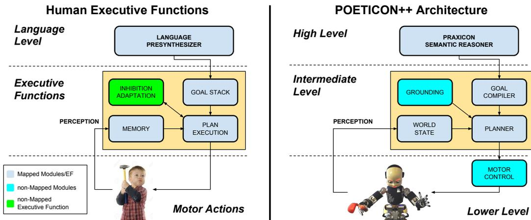
**Figure 2:** Mapping between human EFs (left), and the modules developed for the POETICON++ project (right). Boxes in gray correspond to the EFs mapped to robot modules; light blue (Grounding and Motor Control) corresponds to extra modules not related to EFs, and; green (Inhibition/Adaptation) corresponds to EFs not mapped directly to robot modules. It should be noted this executive function was implemented as a heuristic in the Planner module.
