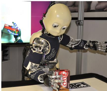
Fig. 1: The iCub humanoid robot performing a precise grasping task by markerless visual servoing.
