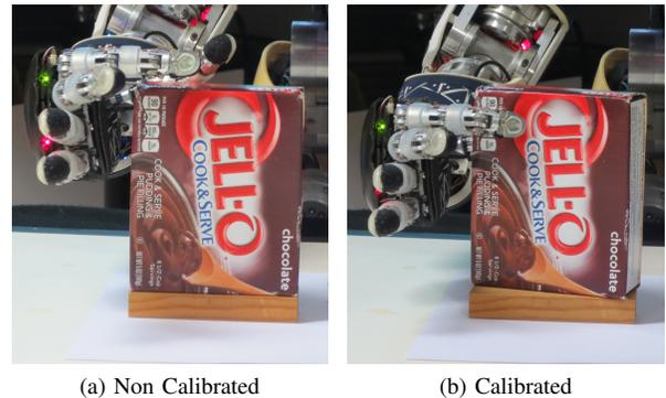
Fig. 4: Example of the final pose of the hand in one of the experiments: uncalibrated (a) and calibrated (b). In the non-calibrated scenario the grasping fails. The desired position for the index fingertip is the lower part of the J on the cover of the JELL-O Pudding Box.
