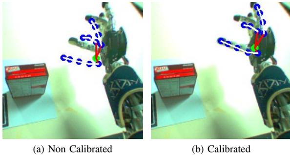
Fig. 3: Example of an uncalibrated (a) and calibrated (b) eye-hand kinematic chain and the errors in the 2D projection of the thumb, index and middle fingers
