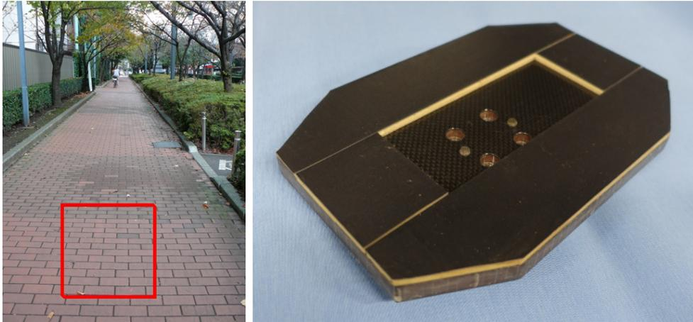
Fig. 3.7 Left: example image from the GTF dataset overlaid with a red square indicating where the coefficient of friction was measured. Right: sole of the humanoid robot foot used for the coefficient of friction experiments, GTF dataset.
