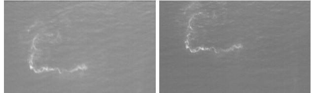
Figure 6: Misalignment of the images for different frequencies due to the UAV motion. On the left is the image for frequency #0 (632.4 nm) and on the right for frequency #15 (680 nm). The luminance of the images was increased in order for the pollutant to be seen.
