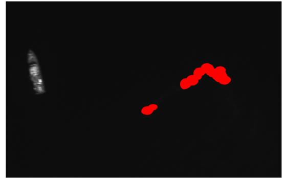
Figure 15 – The result of using the luminance mask. The oil spill is correctly detected and the boat is ignored.
