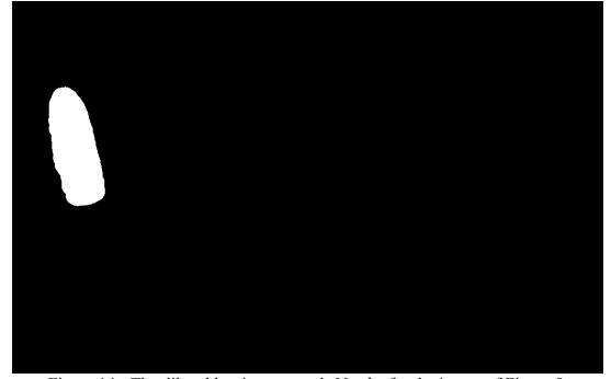
Figure 14 - The dilated luminance mask  $Mask_Y$  for the image of Figure 9.
