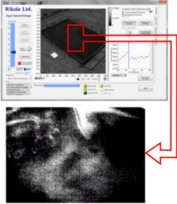
Figure 5: Hyper-spectral camera usage in laboratory tests (fish oil spills in tank)
