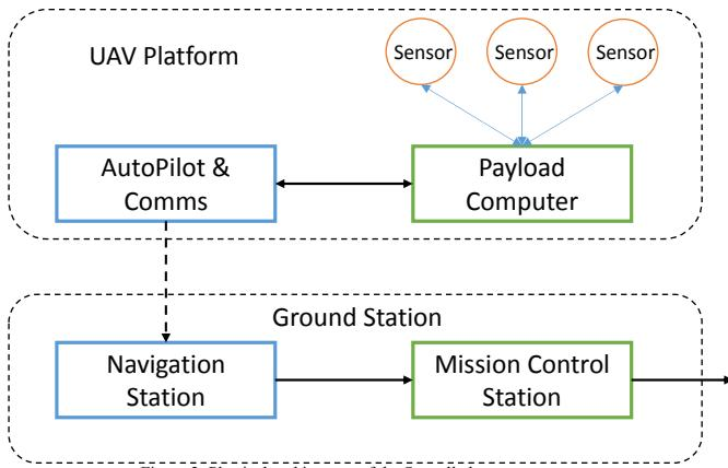
Figure 2: Physical architecture of the Seagull elements.
