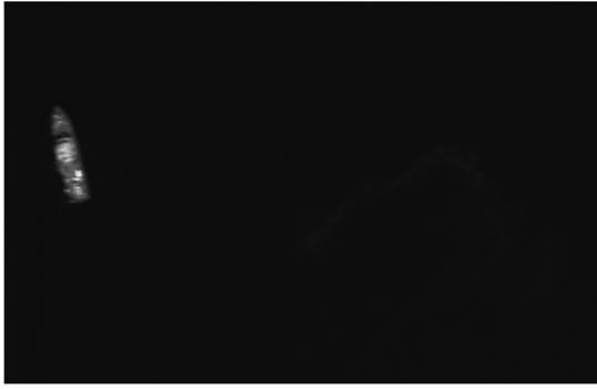
Figure 13 – An image containing a boat. There is also a pollutant spill (similar to the one in Figure 6) on the right side of the image that cannot be seen because the boat luminance is much larger. The pollutant is so dark compared to the boat that becomes indistinguishable from the background.
