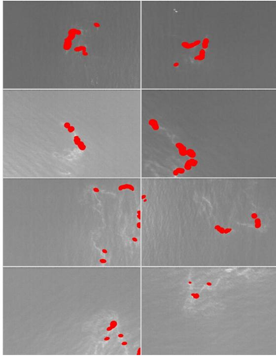
Figure 16 - Detections (marked in red color) obtained for several example image frames. The brightness of the images was increased in order for the oil spills to be clearly visible.
