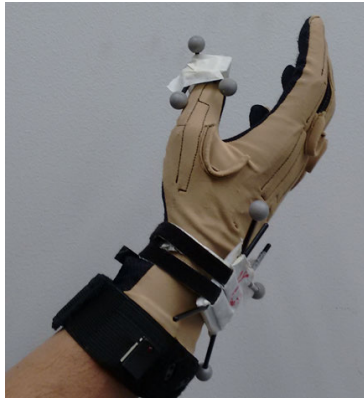
Figure 3.5: Optical markers are used to track the 6D position and orientation of the thumb-tip during thumb workspace exploration.
