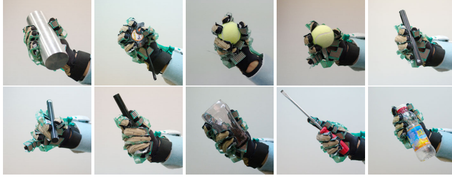
Figure 3.20: Grasp scenarios in Table 3.1 demonstrated on objects using the tactile glove.
