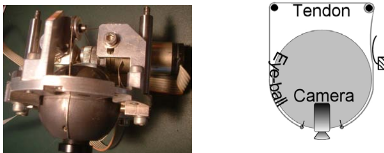
Figure 3.3: The left picture shows one of the eyes and the actuation system. The two tendons are actuated by two motors. The first motor moves the vertical tendon (tilt motion). The second motor moves the horizontal tendon (pan motion). The right figure sketches the actuation scheme, concerning just the pan rotation.
