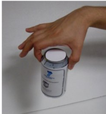
Figure 5.32: First initial grasp of the list: number 9, Palmar Pinch.
