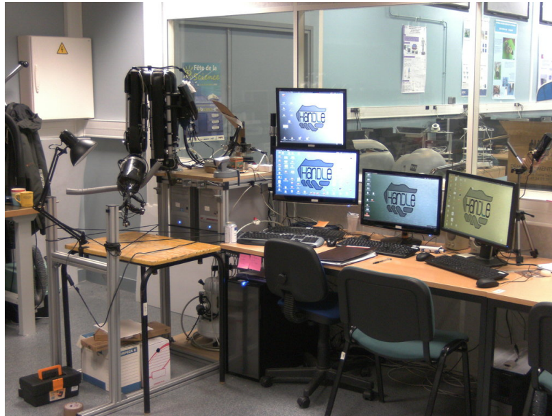
Figure 5.18: The experimental platform: the Shadow hand and arm, mounted on a support structure. The different computers controlling it are visible.
