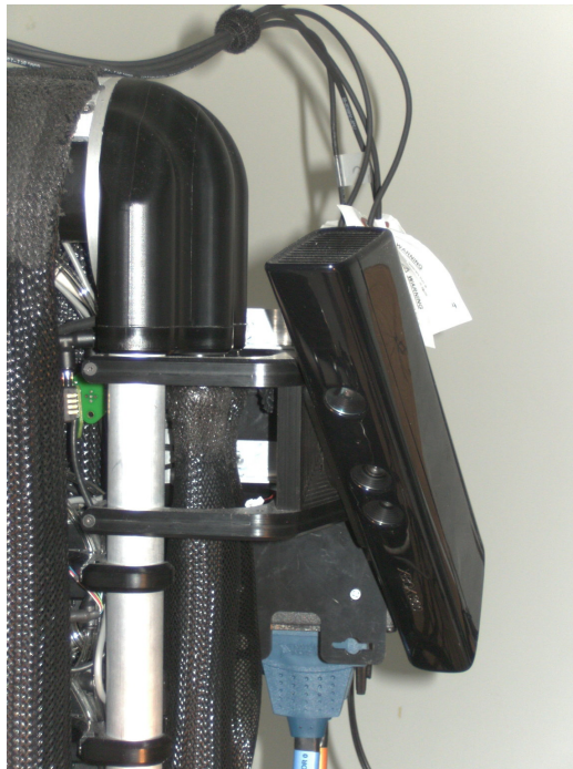
Figure 5.24: The Kinect is mounted on the side of the shoulder.
