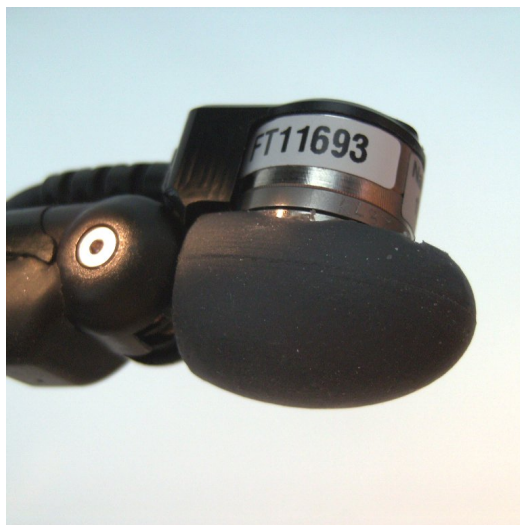
Figure 5.22: ATI Nano17 sensors with ellipsoid rubber fingertip.
