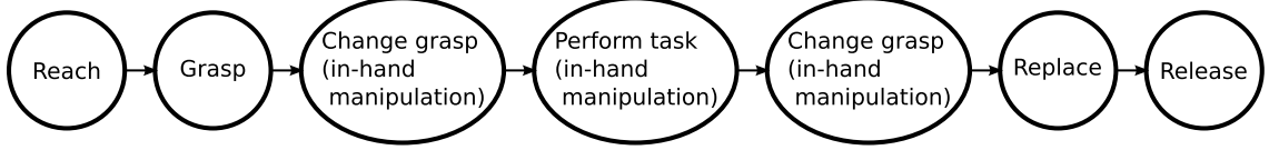
Figure 2.1: Phases during a complete manipulation activity.
