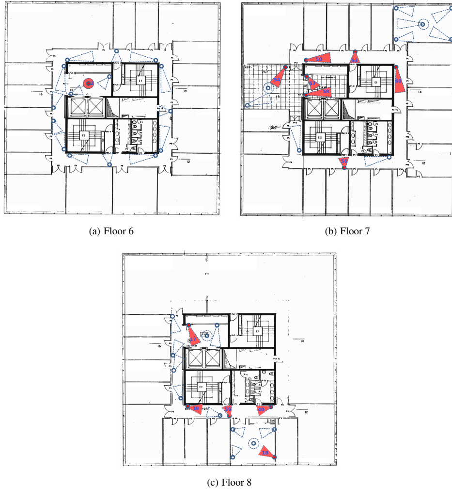
Figure 1 Camera poses: the cameras marked with a red circle and an orange field of view are the cameras used to acquire data.
