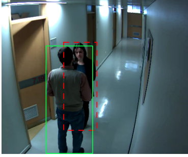
Figure 4: An example of geometrical reasoning: two detection Bounding Boxes overlap. The comparison between the lower sides of the two Bounding Boxes leads to the conclusion that the person marked with the red, dashed Bounding Box is occluded by the person in the green, continuous Bounding Box.
