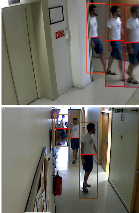
Fig. 1. Two camera views, with several detections, waist-separated, and two tracks. A correct re-identification would cluster them together or label them as the same individual from a database.
