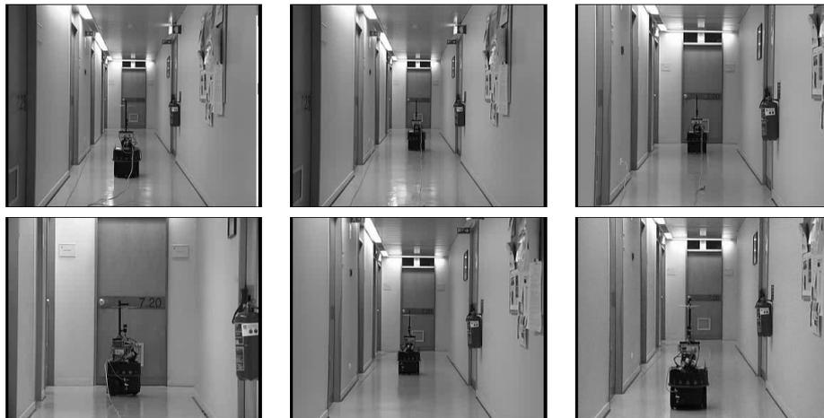
**Fig. 4.8:** A sequence of images of the SCOUT mobile robot navigating in a typical indoor environment.
