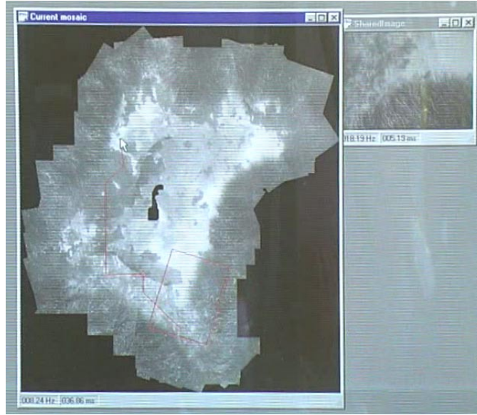
Figure 1.2: Screen capture of the man-machine interface used for navigation. It contains the mosaic map (left) with the estimated position (red rectangular frame), specified end position (arrow) and trajectory. The live camera feed is shown in the upper right window.
