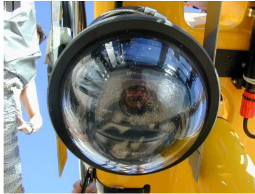
Figure A.3: Close-up on the video camera housing with spherical dome.
