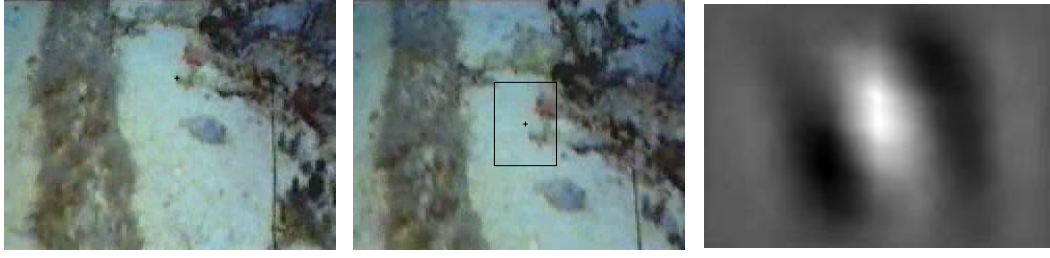
Figure 4.3: Search area selection: image I_1 (left) with selected feature, search area on I_2 (center) and cross-correlation image(right)
