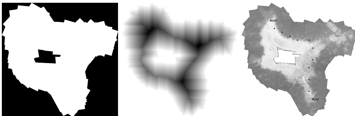
Figure 6.4: Trajectory generation example – Valid mosaic region in white (left), cost image (center) and mosaic with superimposed trajectory (right). In the cost image, the darker regions have lower cost.
