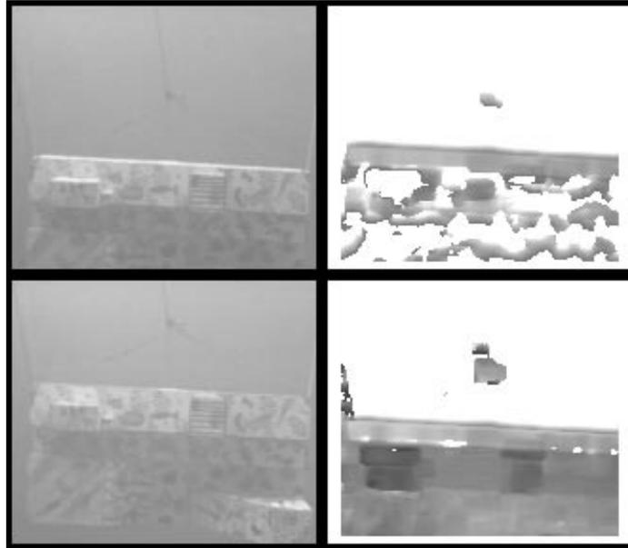
**Figure 2.10:** Left : Underwater stereo image pair. Right : The top image shows the depth map recovered using the equalization procedure, while the lower image corresponds to the results using equalization.
