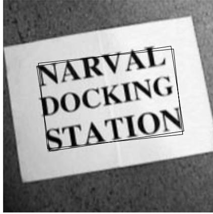
Figure 3.9: ROI position in target image as predicted by the difference template method. Also the initial prediction was super-imposed.
