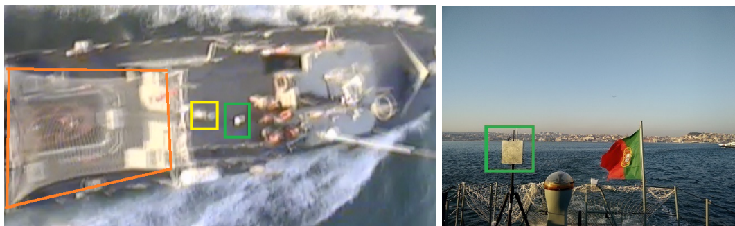
Figure 2.3: Landing area ( orange ), RGB camera ( yellow ), and communications ( green ).
