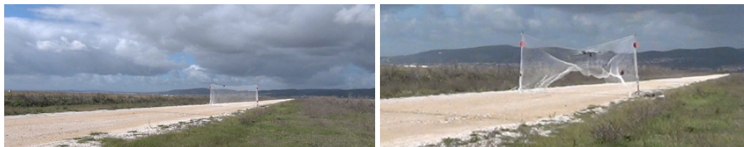
Figure 2.2: Net-based retention system ( experimental test example ).
