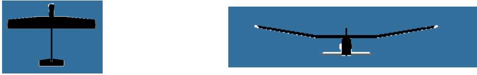
Figure 6.17: An example of 180 degrees variation on Z (left) and 180 degrees variation on Y (right) where the black color corresponds to the pose overlap.
