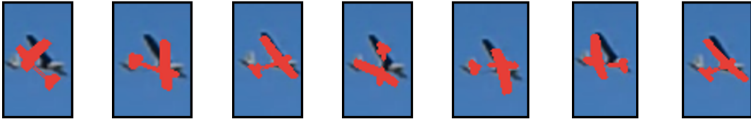
Figure 4.7: Observation frame OBB detection. From left to right: (i) original image, (ii) detected ROI , (iii) FAST features, and (iv) OBB .
