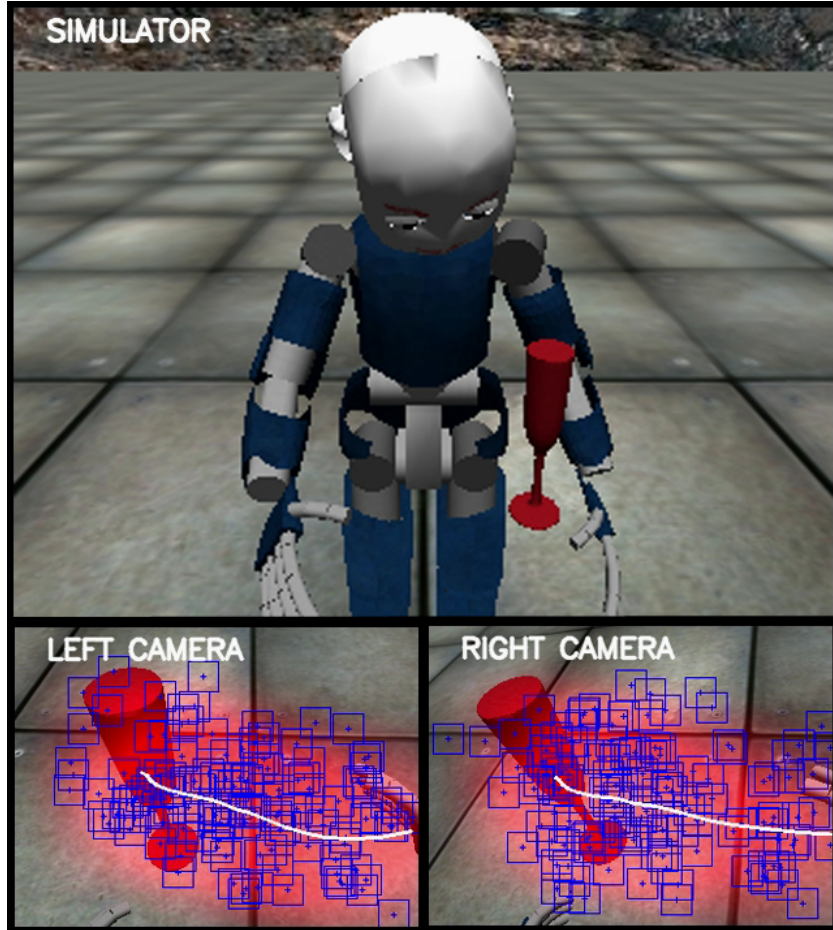
Figure 5.2: The figure displays the main idea of the proposed approach: nonuniform image processing driven by a motor-primed visual attentional landscape. Visual space is prioritized depending on its motor relevance; i.e., visual attention is biased toward motor-relevant parts of the workspace projected to the stereo images. The white line represents a forward-planned (mentally-simulated) movement toward the object to be grasped (red glass). The reddish blend superimposed on the snapshots of the left and right cameras is a visualization of the intensity of the visual attentional landscape. The attentional landscape has a higher intensity closer to motor relevant parts of the visual field. The images are processed in a manner that the spatial distribution of their attentional landscapes is taken into account (motor-relevance is prioritized). The anchors of the scanning windows (blue squares) are sampled with respect to their relevance, i.e. more dense visual scanning is done where the attentional landscape has higher values, and less dense scanning where it has low values. Ignoring irrelevant parts of the images affords significant computational savings, whereas the processing of motor-relevant parts of the visual scene supports visually-guided reaching and grasping.
