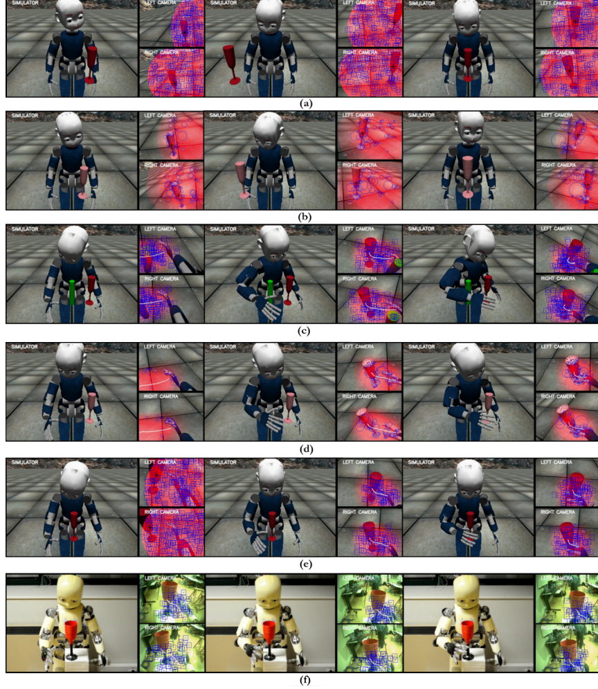
Figure 5.6: Experiments of visual exploration for object detection (a-b) and visually-guided reaching and grasping in the iCub’s simulator (c-e), in two different scenarios with two detectors, and the real robot (f). The reddish blend shows the superimposed attentional landscape used to drive visual processing (for the peripersonal space-primed attention with the histogram-based detector (a) we are sampling from a modified version, computed as in Eq. 5.10 with \pi = 0.2 ). The figures (a) and (b) represent snapshots from the experiments where visual processing is prioritized to the peripersonal space (peripersonal space-primed attention), for histogram-based detector and SURF, respectively. The blue squares are scanning image windows for which visual features are computed. The robot adopts a random configuration, and the object adopts a random position within the reachable space. Figures (c-f) show the context of motor plans-primed attention, namely, the execution of eye-arm-hand coordination from the start of the task (left) until successful grasp completion (right). The white line corresponds to a mentally-simulated arm trajectory that is projected to the image planes of stereo cameras. Figure (b) corresponds to the obstacle scenario with histogram-based detector. Figure (c) corresponds to the obstacle scenario with histogram-based detector. Figure (d) corresponds to the no-obstacle scenario with SURF detector. The blue circles correspond to detected strong feature points. Figure (e) shows how a combination of both approaches: the peripersonal space-primed attention is used to bootstrap initialization of the motor plans-primed attention. The bottom row (f) corresponds to the no-obstacle scenario with histogram-based detector with the real robot.
