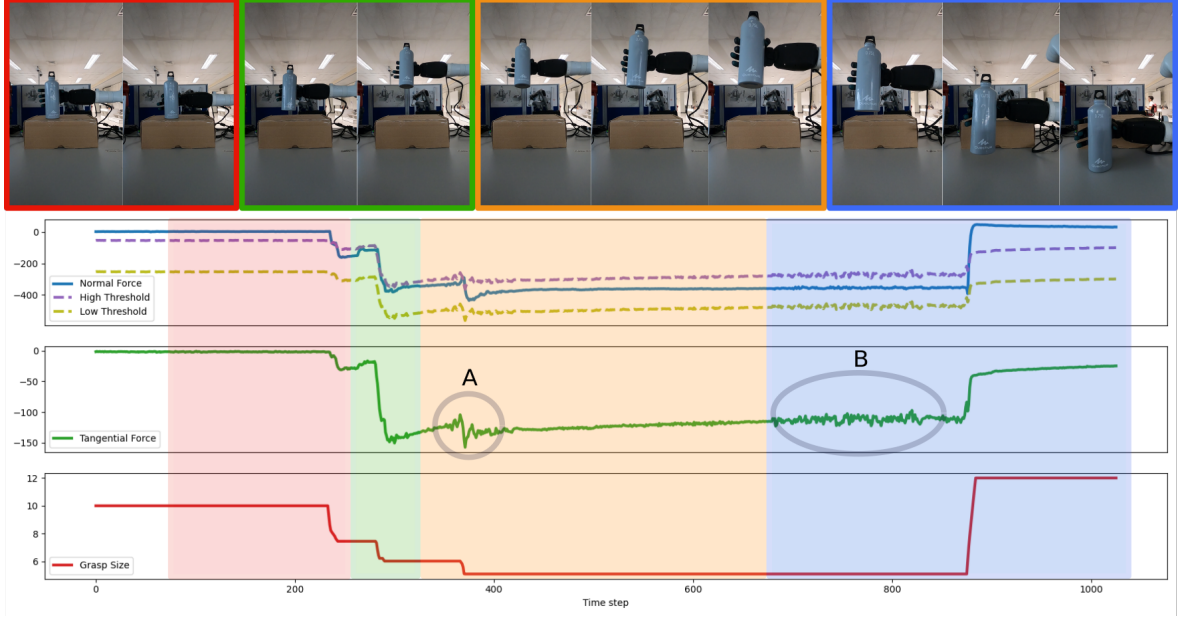
Figure 4.7: In our first experiment, the robot grasps and lifts a bottle, transports it, and places it on the desk. The bottom part of the figure shows see the control signals recorded during this task.
