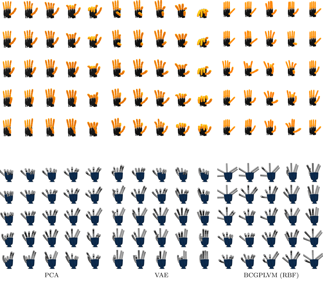
Figure 3.6: Grasp postures decoded from the a regular 5 \times 5 grid in the 2D latent spaces of three models: PCA (first column), VAE (second column), and BCGPLVM (RBF) (third column). The first row contains grasp postures using the Shadow Hand and the second row using the iCub hand.
