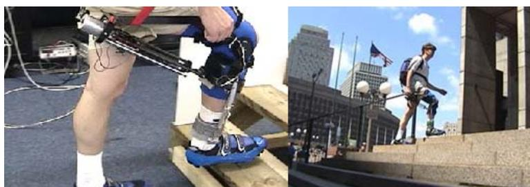
**Figure 4:** RoboWalker, an example of a robotic prostheses
