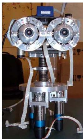
**Figure 22:** Prototype of robot head with spring-based neck, produced by University of Genoa
