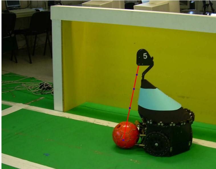
*Figure 5.1: Initialization of the filter: particles are spread along a 3D ray based on a couple of image coordinates selected by a detection algorithm. The distribution used to initialize the filter will be Gaussian, centered on the particle, among the ones spread along the ray, with the highest likelihood.*
