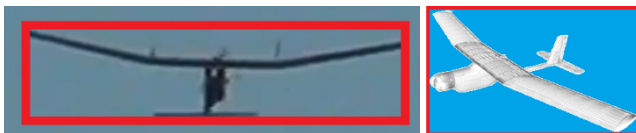
Figure 3 Example of object inner (object) and outer (between the object and the bounding box) regions where color histograms are computed for the particle likelihood metric.
