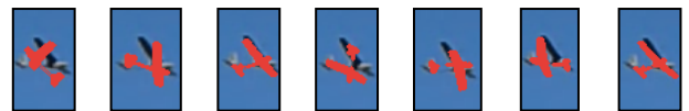
Figure 9 In red we can see the projection on the real image of randomly selected possibilities for particle initialization from the best database matches.
