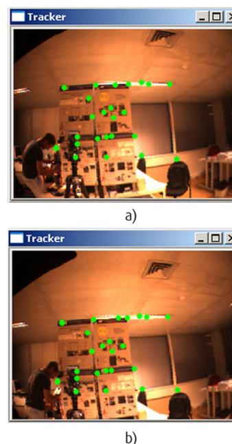
Figure 5 · Right eye image grabbed with tracked points, before (a) and after (b) the tilt motion.
