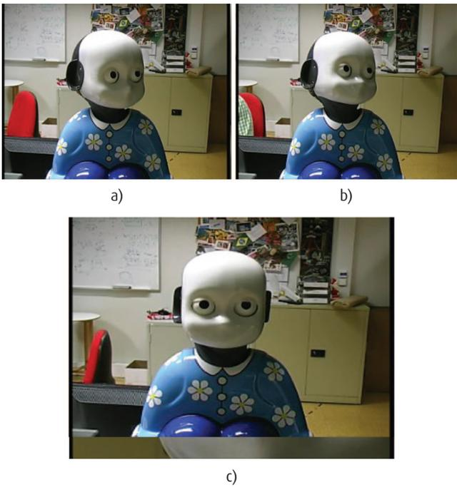
**Figure 6** · Calibration procedure for the neck pan. The robot starts up with significant offset in the neck pan joint, with respect to its canonical position (a). A motion of 10 degrees is applied to the neck tilt (b). The proposed method estimates the initial pan angle and compensates it (c).
