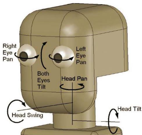
Figure 3 · Kinematics of the iCub robot head used in the tests.
