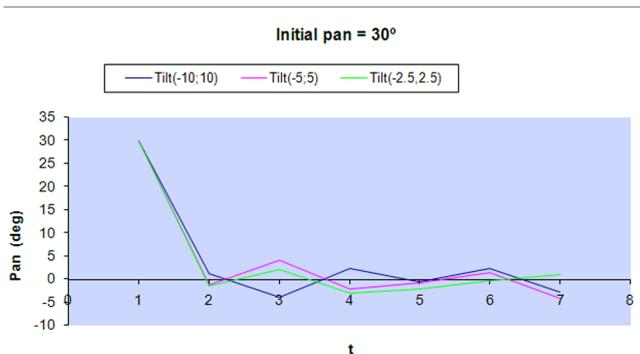
**Figure 7** · Evolution of the pan angle for an iterative application of the calibration method. Different colors represent different prospective motion amplitudes.
