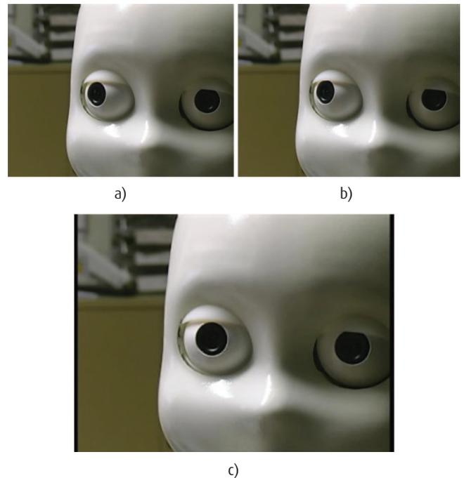
Figure 4 · Sequence of motions required to calibrate the eye. a) right eye position at startup. b) right eye position after prospective tilt motion. c) right eye position after calibration.
