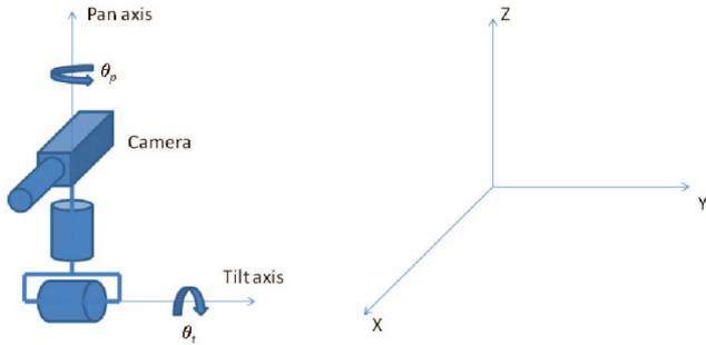
**Figure 1** · Left: the kinematics structure of the pan-tilt system considered in this paper. Right: the adopted orientation for all the involved coordinate frames.
