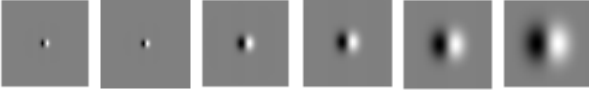
Figure 2: Examples of odd Gabor functions at \theta = 0 , \gamma = 6 , and \sigma = \{2\sqrt{2}/3, 4/3, 4\sqrt{2}/3, 8/3, 8\sqrt{2}/3, 16/3\} .
