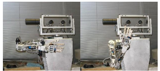
Fig. 1. Sensory-Motor Coordination learned by self-exploration. The redundancy of robots make it harder to associate perception to actions.
