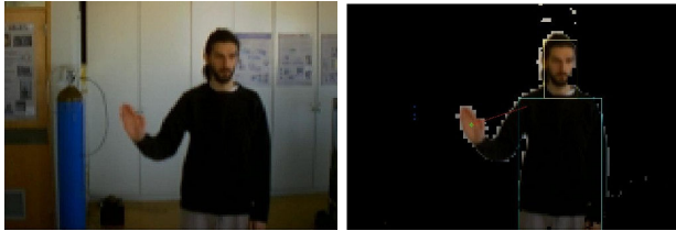
Fig. 12. Vision system. Left: original image. Right: background segmentation of the human figure and hand detection. The rectangular frame is used for the template matching.
