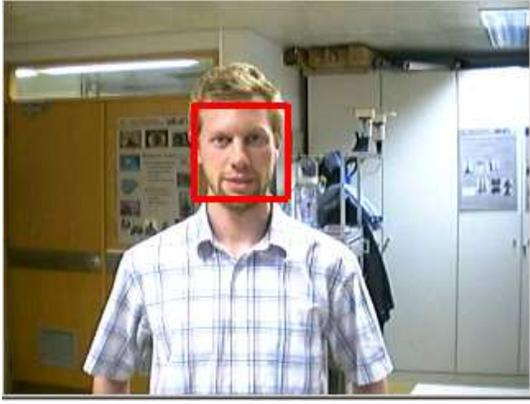
Fig. 9. Result of the face detection algorithm used as a feedback signal for the sound localization algorithm.
