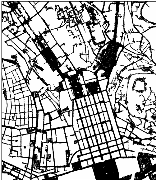
Figure 2 – Result of region growing on the DSM. Dark areas correspond to the roads and ground plane regions. Bright areas correspond to buildings, trees and other above ground structures.
