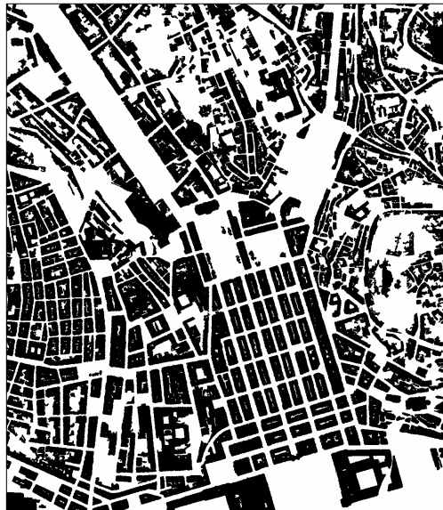
Figure 4 – Building Segmentation. Dark areas correspond to blocks of buildings, with high likelihood.
