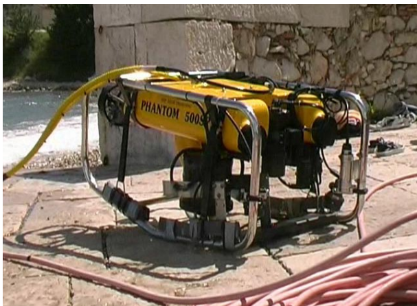
Fig. 6. Computer controlled Phantom ROV with the on-board camera. The camera housing is visible in the lower center, attached to the crash frame.
