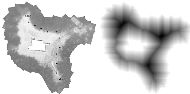
Fig. 3. Trajectory generation example – Mosaic with superimposed trajectory (left), and corresponding cost image (right).
