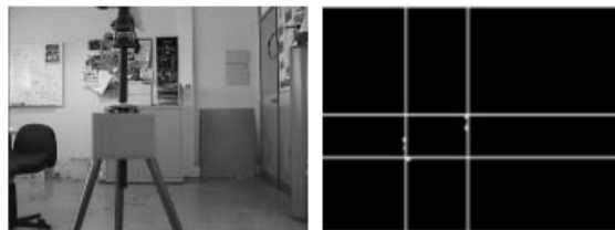
Figure 1: Detection of the blue rectangle’s corners for the following behaviour.
