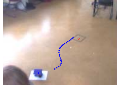
Figure 7: Example of robot trajectory superimposed on the image.
