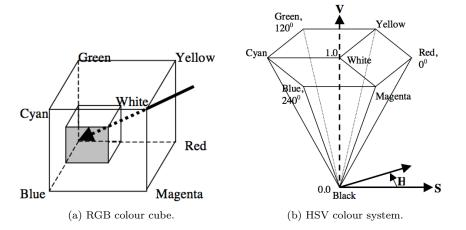
Figure 4.2: RGB and HSV colour spaces. In the single-hexcone HSV model, the V = 1 plane contains the RGB model's R = 1, G = 1, and B = 1 planes in the regions shown.
