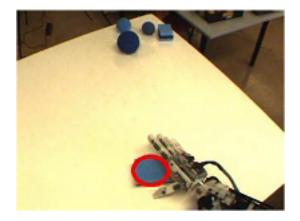
Figure 1.3: Humanoid robot Baltazar operating in its workspace, as seen from one of its cameras. The anthropomorphic hand of Baltazar is reaching for a visually-tracked object and is about to grasp it.
