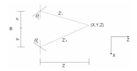
Figure 4.5: 3D reconstruction scheme for a stereo pair of cameras with arbitrary vergence.
