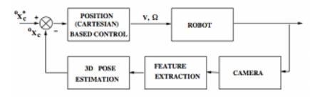
Figure 2.18: Block diagram of PBVS [HHC96]. The estimated pose of the target,  ${}^{c}\mathbf{x}_{0}$ , is compared to the desired reference pose,  ${}^{c}\mathbf{x}_{0}^{*}$ . This is then used to estimate the velocity screw,  $\dot{\mathbf{q}} = [\mathbf{V}; \mathbf{\Omega}]^{T}$ , for the robot so to minimize the error.
