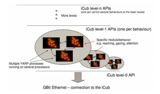
Figure 3.11: Software architecture of the iCub (and RobotCub).
