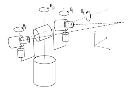
Figure 3.3: Scheme of Baltazar robotic head, code-named "Medusa" [BSV99]. The meaning of the four joint angles  $\theta_l, \theta_r, \theta_p$  and  $\theta_t$  is explained in Table 3.1.
