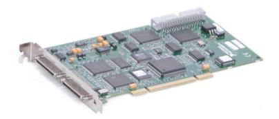
Figure 3.10: National Instruments 7340 Stepper/Servo Motion Controller.
