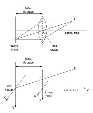
Figure 4.4: Pinhole camera model.
