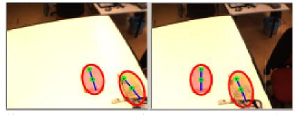
(a) Object and hand are parallel;  $\mathbf{u} = (X = -0.006, Y = -0.062, Z = -0.041), \theta = 4.285^{\circ}$ .
