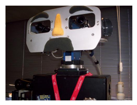
Figure 3.4: Real Baltazar robotic head.
