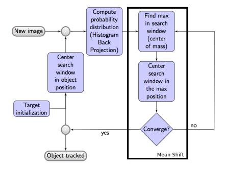
Figure 4.1: Block diagram of CAMSHIFT.
