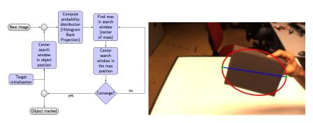
Fig. 2. Left: Flux diagram of the CAMSHIFT object tracking algorithm. Right: CAMSHIFT tracking of an object. The approximating best-fit ellipse is drawn in red, the major axis in blue, and the extremities of the axis are small green circles.
