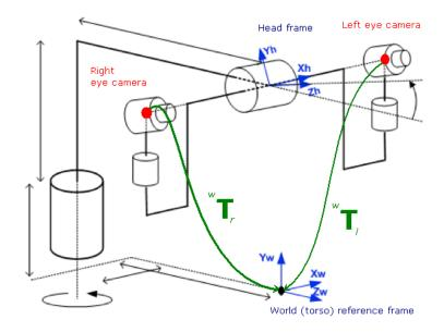
Figure 4.7: Mechanical structure of Baltazar head, its reference frames and points of interest. Transformation matrices are highlighted in green.
