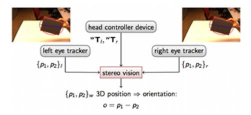
Figure 4.6: 3D reconstruction software module scheme, outlining the data that are passed as inputs/outpus among YARP modules.
