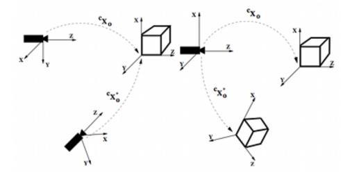
Figure 2.17: Two examples of PBVS control. Left: eye-in-hand camera configuration, where the camera/robot is servoed from  ${}^{c}\mathbf{x}_{0}$  (current pose) to  ${}^{c}\mathbf{x}_{0}^{*}$ (desired pose). Right: a monocular, standalone camera system used to servo a robot-held object from its current to the desired pose.
