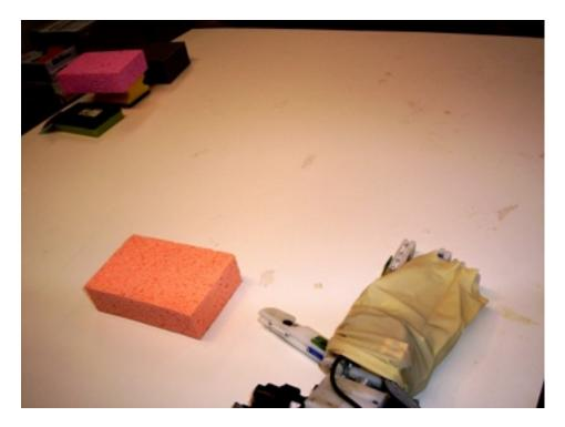
Figure 5.6: Baltazar robot hand wearing a glove, in order to make its colour more homogeneous, thus facilitating CAMSHIFT tracking and 3D reconstruction of the hand.
