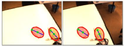
(b) Object and hand have a relative slope of roughly 45°;  $\mathbf{u}=(X=-0.129,Y=0.737,Z=-0.129),\theta=49.413^\circ.$
