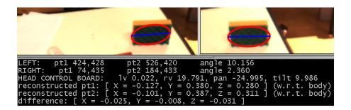
Figure 5.3: 3D reconstruction experiment.
