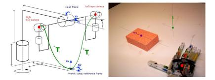
Fig. 3. Left: mechanical structure of Baltazar's head, reference frames and points of interest; transformation matrices are highlighted in green. Right: unit vector of the target object along its orientation axis (purple), versor and orientation of robot hand (red), and third axis resulting from their cross product, and corresponding unit vector (green).
