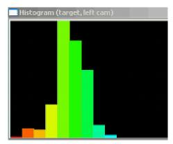
(b) 16-bin CAMSHIFT colour histogram used for iterative searches during all of the experiment of Fig 5.2a.
